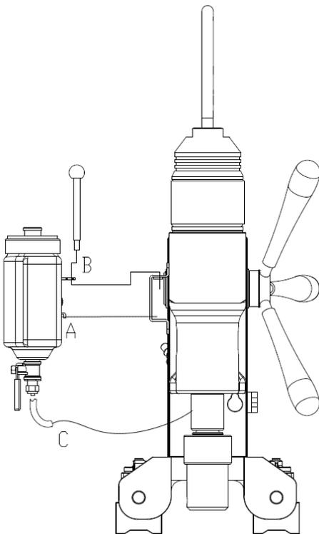
1. Hang the oil tank (A) on the tank holder
